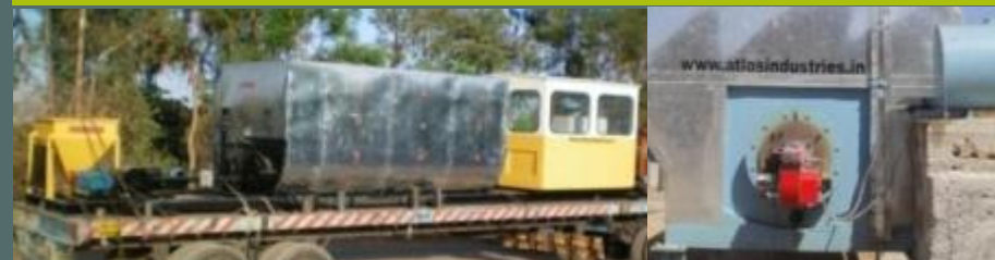
BITUMEN TANK WITH LIME FILLER AND CABIN
