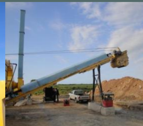
**FULLY COVERED LOAD OUT CONVEYOR TO REDUCE HEAT LOSS FROM HOT MIX
